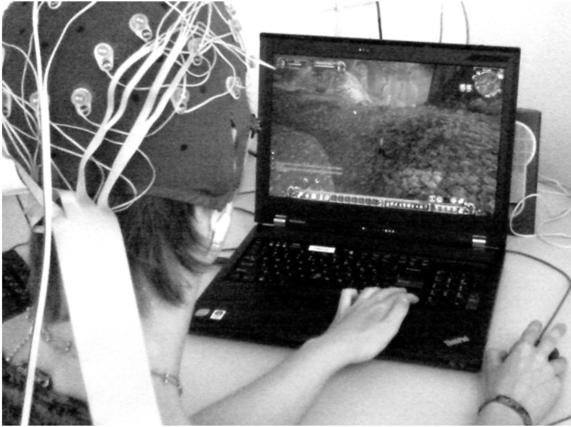
FIGURE 7: Participant playing AlphaWoW: with the Biosemi headset. Mouse and keyboard are still used for movement, selection, and camera control.
