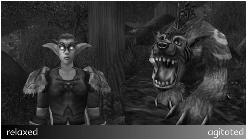
FIGURE 6: BCI control in World of Warcraft®: When the user is relaxed (high parietal alpha activity), the avatar is humanoid. When the user gets agitated (low parietal alpha activity), the avatar becomes a bear.
